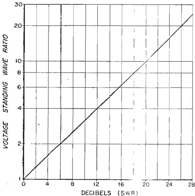
Figure 2-4. Graph Showing Standing Wave Ratio in DB vs. VSWR
