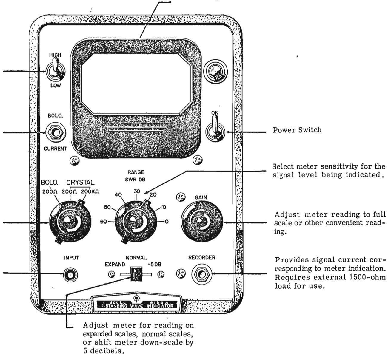
Figure 2-2. Controls and Terminals Diagram
