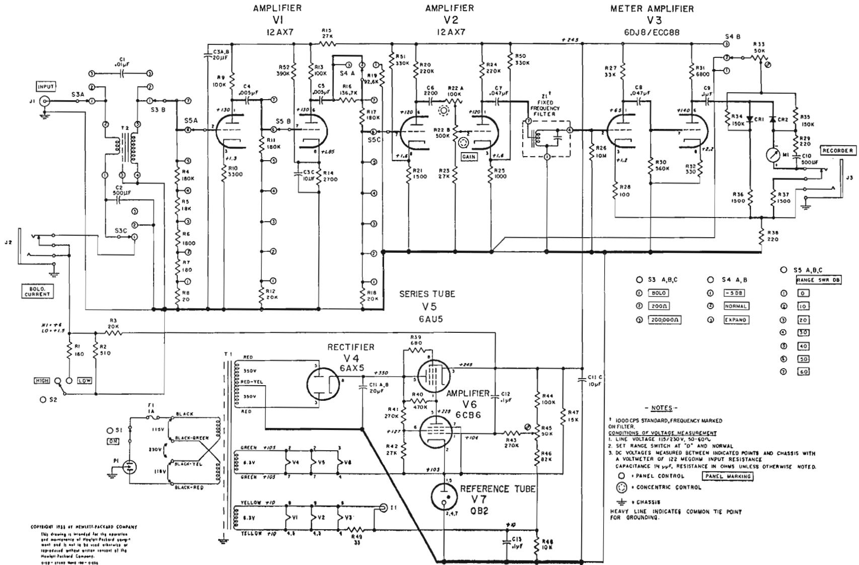
Figure 4-5. Model 415B Standing Wave Indicator
