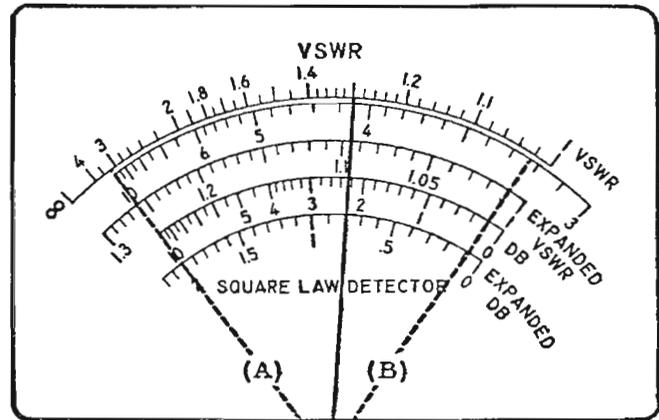
Figure 2-3. Detail of Meter Face
