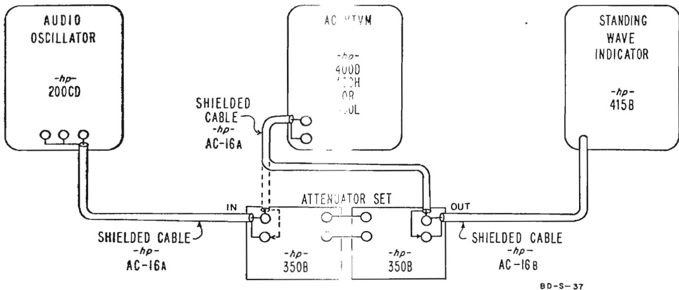
Figure 4-1. Instrument Connections for 415B Test and Adjustment
