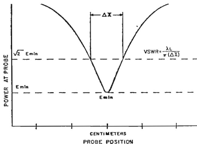
Figure 2-7. Graph Showing Double Minimum Method for Computing VSWR
