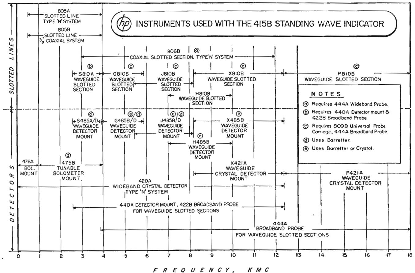
Table 1-1. Suitable Hewlett-Packard Microwave Equipment for Slotted Line Measurement arranged by frequency range
