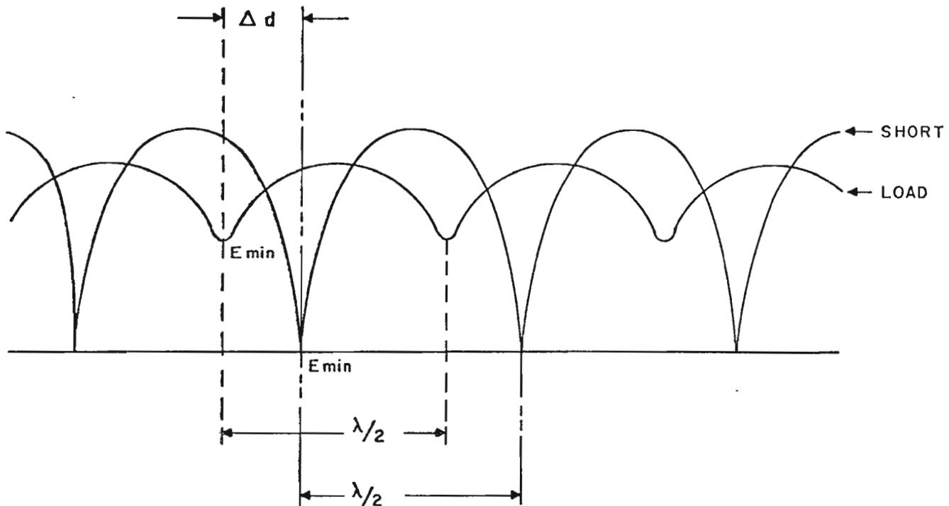
Figure 2-9. Graph Showing Standing Wave Patterns with a Load and Short
