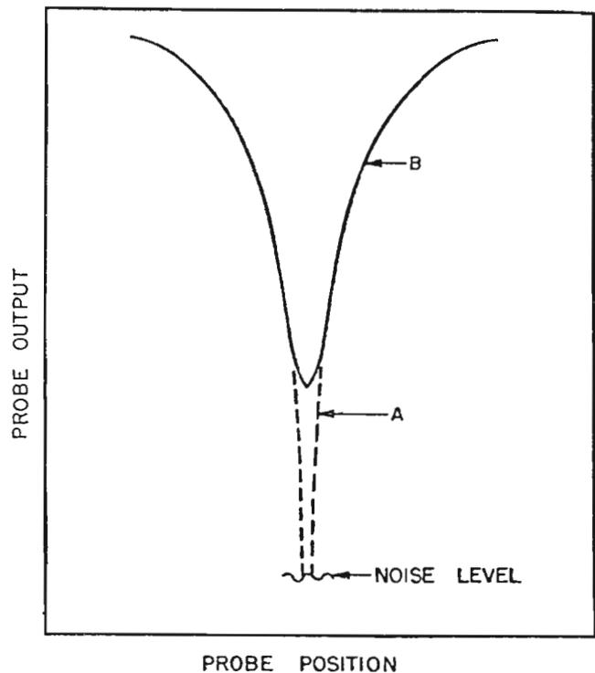
Figure 2-5. High Standing Wave Ratio Pattern
