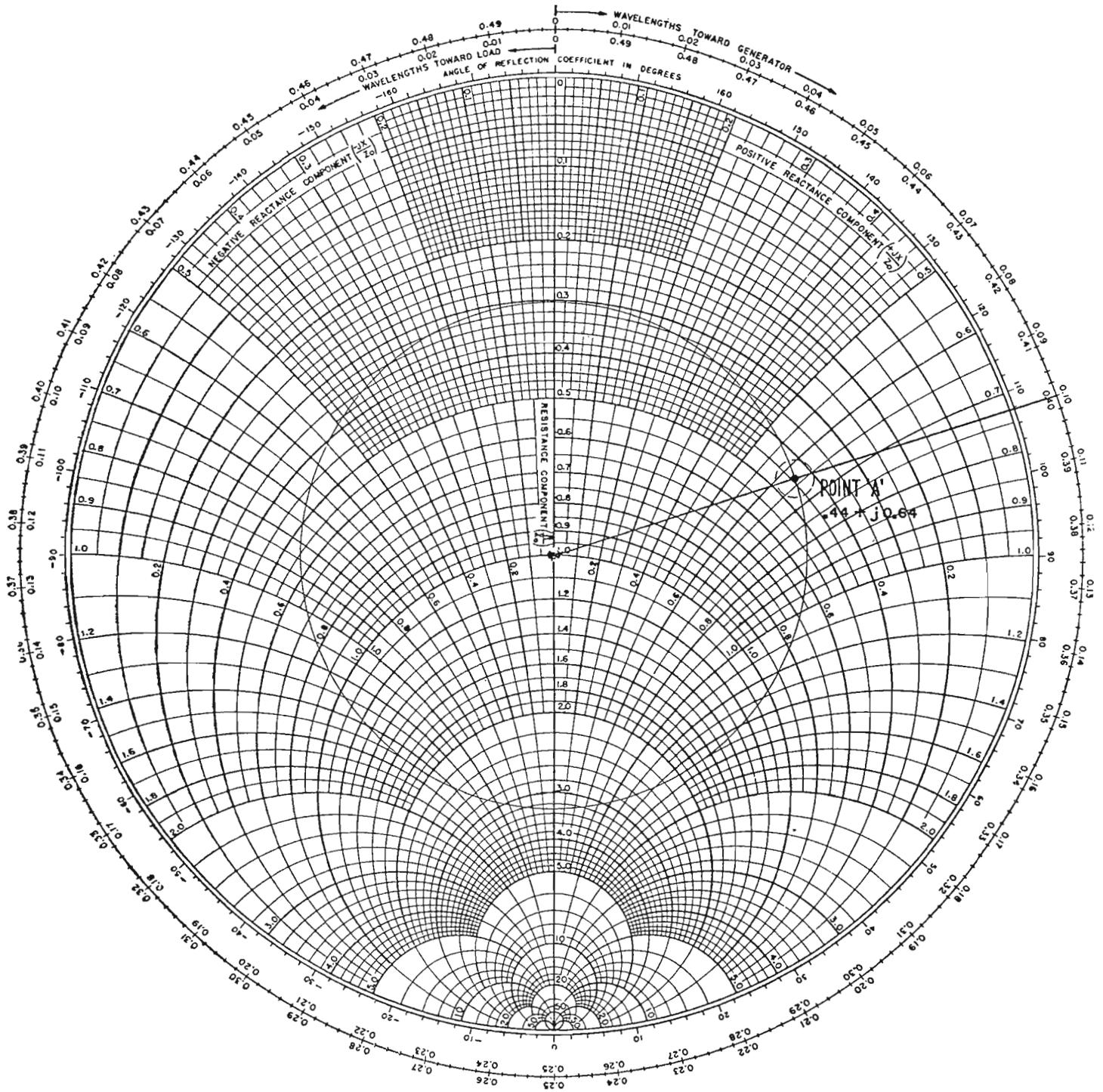
Figure 2-12. Smith Chart Showing Impedance Point,  $\Delta$
