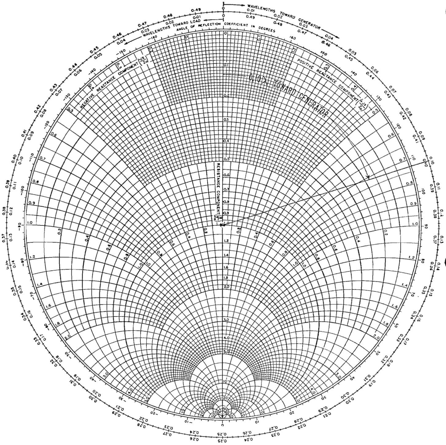
Figure 2-11. Smith Chart with Wavelength Shift Point Constructed as a Radius.  $\Delta \lambda = 0.1$
