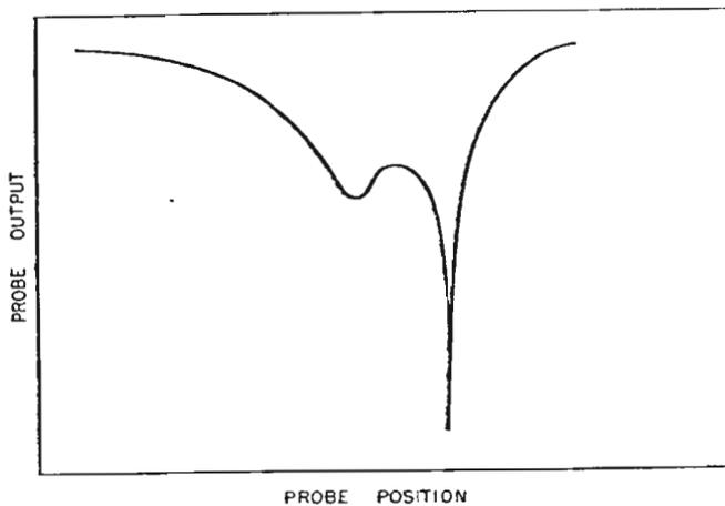
Figure 2-6. Typical Pattern of High VSWR to Spurious Frequency in Signal Source
