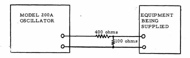
Other values of resistance may be used to obtain different voltage divisions. In all cases, the sum of the divider resistors must equal the rated load of 500 ohms.
