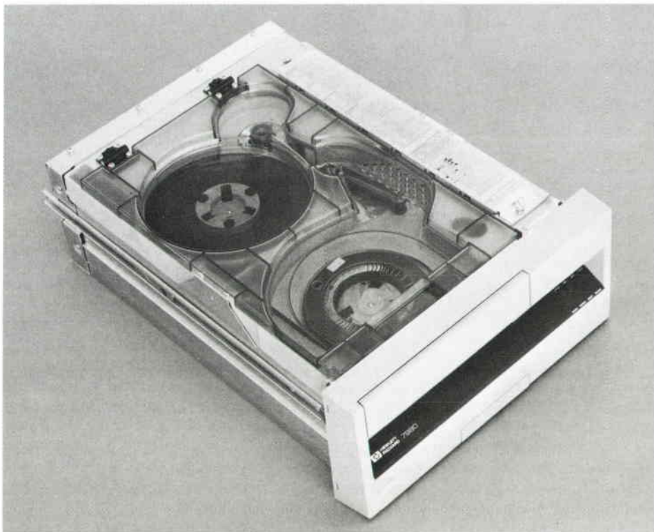
Fig. 1. The HP 7980A Tape Drive is a half-inch, reel-to-reel, 125-ips streaming tape drive designed for systems with disc backup requirements of greater than 400 megabytes. Like its predecessor, the HP 7978B, this high-performance drive operates with both 6250 GCR and 1600 PE standard formats. The HP 7980A can automatically load and thread any size reel ranging in diameter from six to 10.5 inches. This drive can be horizontally mounted in a 19-inch-wide rack enclosure for better floor-space utilization, and it supports IBM/ANSI-compatible formats for software distribution and data interchange between HP and non-HP systems.
