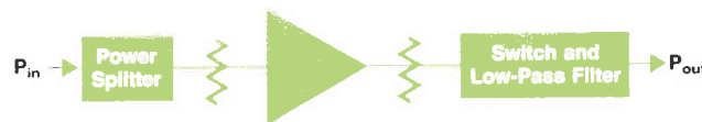
Fig. 1. A typical power path on one board at a single frequency (470 MHz).
