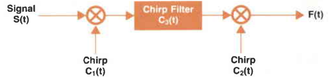
Fig. 4. Chirp filter implementation of analog Fourier transform. Chirps C_1(t) and C_2(t) can be generated by pulsing SAW chirp filters. The output F(t) is the Fourier transform of the signal S(t) .
