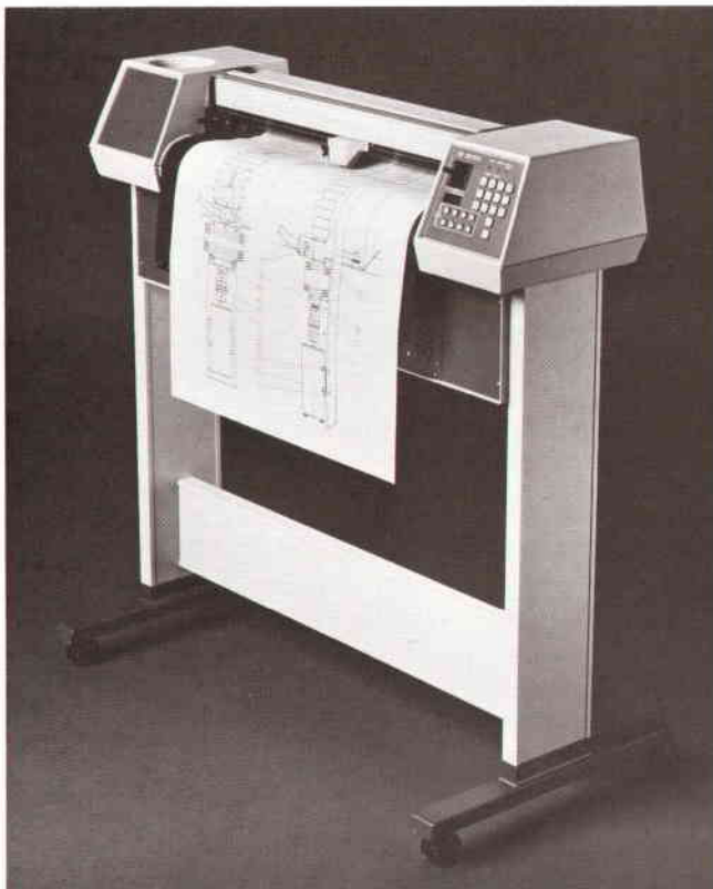
Fig. 1. The HP Model 7580A Drafting Plotter uses a micro-grip paper-drive mechanism to produce high-quality drawings on a variety of commonly used drafting media. Liquid-ink, fiber-tip, or roller-ball pens can be easily used to meet different drafting requirements. The design reduces the cost of the instrument, its power consumption, and the floor space required.
