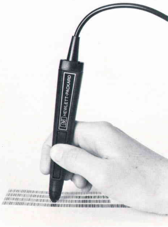
Fig. 1. The 82153 Wand accessory to the HP-41C Calculator provides easy entry of data and programs printed in bar code.
