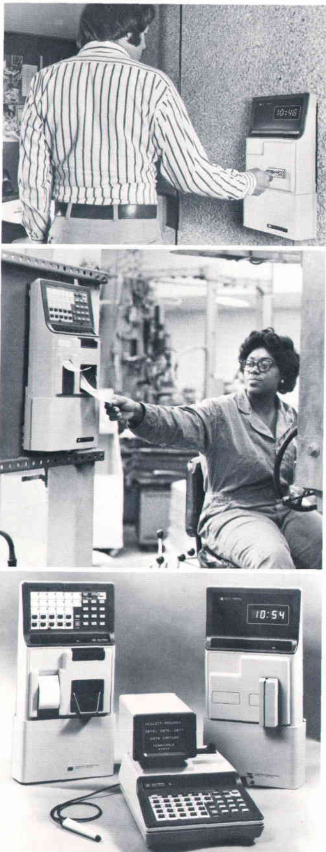
Fig. 2. Data collected by DATACAP/1000 is entered manually by factory personnel using a variety of HP data capture terminals like these.
