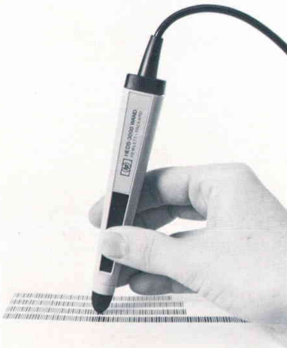
Fig. 1. The HEDS-3000 Digital Bar Code Wand contains all of the components necessary to convert a printed bar-code pattern into a digital signal for use in data processing.
