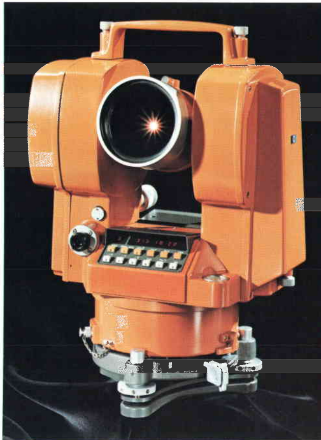
Fig. 1. Model 3820A Electronic Total Station. This instrument combines electronic distance and angle measurement capabilities into a compact package. The values obtained with the 3820A are accurate to a few millimetres for distances up to five kilometres and to a few arc seconds for horizontal and vertical angles.
