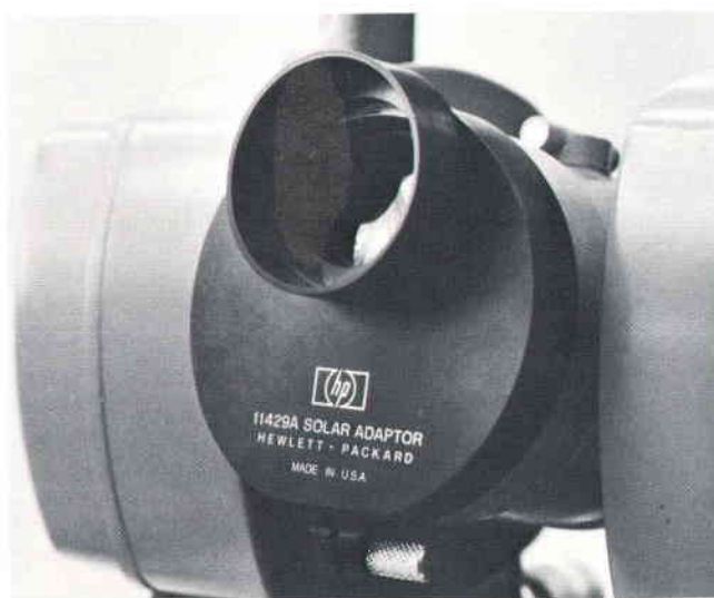
Fig. 3. Roelof's Solar Prism Adaptor. This accessory for the 3820A allows measurement of the angle of the sun above the horizon.
