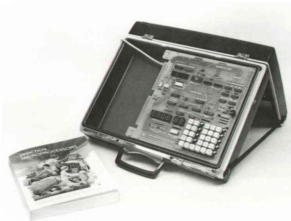
Fig. 1. Model 5036A Microprocessor Lab includes a keyboard-controlled microcomputer and a comprehensive textbook that contains both text and experiments.
