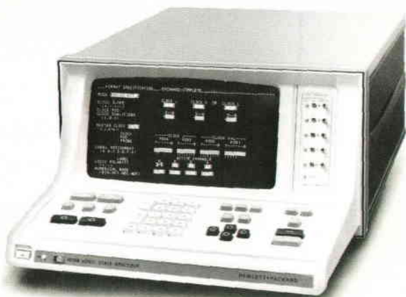
Fig. 1. Model 1610A/B Logic State Analyzer traces the flow of simultaneous digital events in as many as 32 bus lines in digital systems at clock rates up to 10 MHz. Its selective triggering capabilities enable it to restrict data capture to specific loops or branches in complex programs. Keyboard control and an interactive display that uses menus enable rapid set up of complex measurement parameters. The Model 1610B shown here can have data strobed in by three different clocks.
