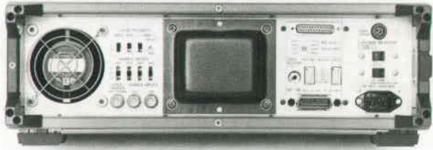
Fig. 8. The ENABLE SELECT switches and two of the four ENABLE inputs are on the rear panel. Also on the rear panel are the LOGIC POLARITY switches, DAV DELAY adjustment, RS 232C BAUD RATE select, and HP-IB addresses ( KEYBOARD and DATA MODES ).
