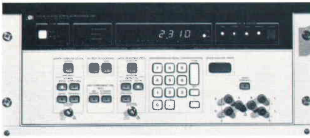
Fig. 1. Front panel of analog stimulus/response unit enables manual control of test procedures. The digital displays show instrument status and also provide diagnostic messages during troubleshooting.
