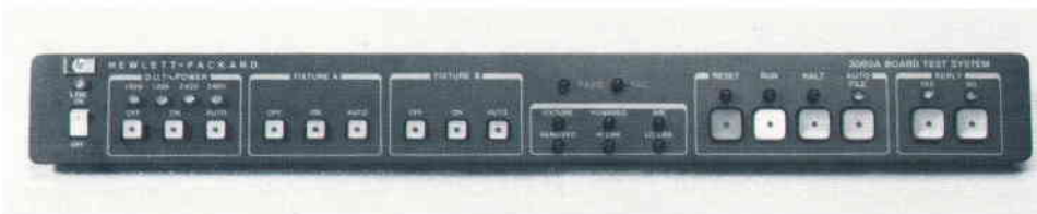
Fig. 2. Board test system control panel, adjacent to the test fixture, has pushbuttons that handle all the testing operations, and indicators that show system status.
