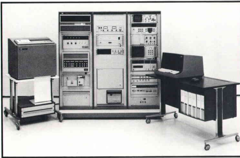
Fig. 1. 9550 Instrument Calibration Systems are modular computer-controlled dedicated systems designed to help solve calibration laboratory problems of work overload, personnel training, and laboratory management. Large and small systems are available. Calibration-quality stimulus and measuring instruments, plus computer-applied corrections, assure that automated calibrations equal or exceed manual methods.
