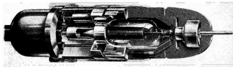
Figure 1. Construction details of new *-hp-* diode probe
