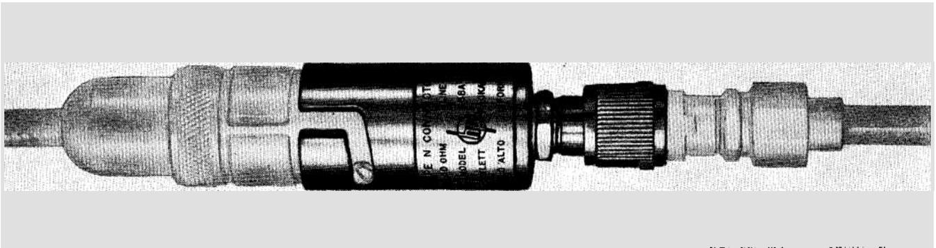
The *-hp-* 458A Type "N" Connector is designed for use with the *-hp-* 410A Vacuum Tube Voltmeter. It is used to connect the special diode probe of the *-hp-* 410A Voltmeter to the open end of a 50 ohm coaxial transmission line. (No terminating resistor is included.)
