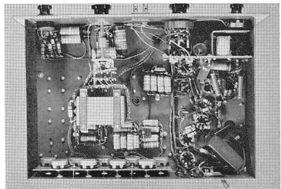
regulated power supply is built into the instrument to minimize the effect of line voltage fluctuations.
