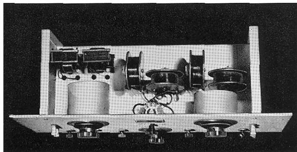
be analyzed adjusted to the proper frequency the fundamental is eliminated completely. The residual voltage containing the harmonics can then be observed with an oscilloscope or measured with a sensitive meter. When the frequency has been adjusted so the fundamental is eliminated, the elimination filter is switched out and a calibrated attenuator is introduced.
