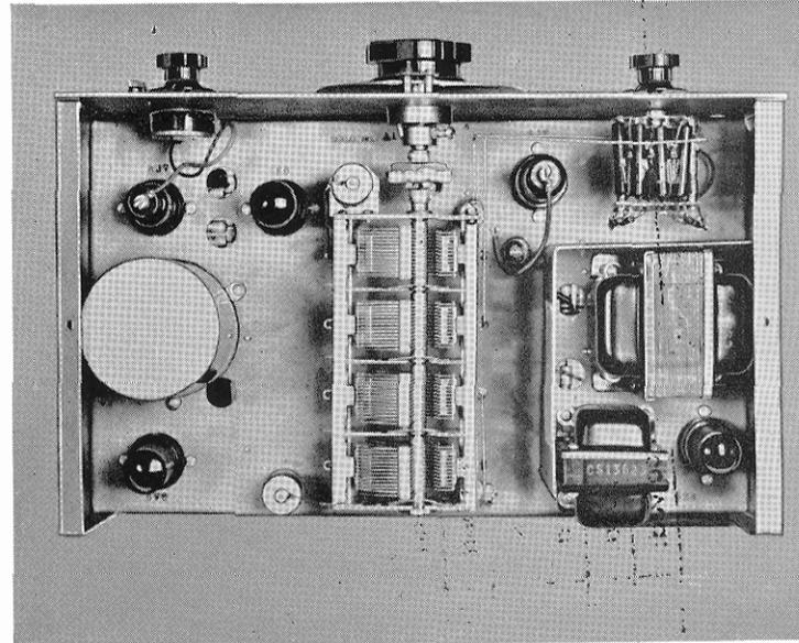
Thermal drift is kept at a minimum by low temperature coefficient elements in the resistance network. The frequency is tuned over a 10 to 1 range by means of the variable condenser. The range is multiplied by selection of the proper resistor with the panel switch.
