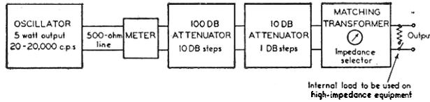
an impedance matching transformer is provided to match various impedances. The output transformer has the same insertion loss for all impedances and the output meter is arranged to read the output voltage at the output terminals with the system loaded. An internal load is provided so the attenuation system works correctly when there is no external load.
