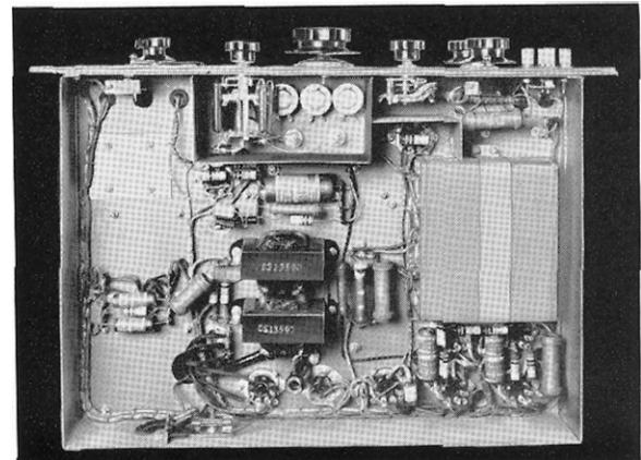
oscillator has a five-watt output which feeds directly into a 500 ohm line where the voltage is measured. The amplitude of this voltage can be set to any level up to plus 37 decibels above one milliwatt by means of the amplitude control on the oscillator. Following the meter are two attenuators, one providing 100 decibels in 10 decibel steps and the other providing 10 decibels in 1 decibel steps. From the output of the attenuators
