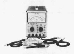
A shock hazard may exist in units with serial numbers 0982A22339 thru 0982A22718. These voltmeters may have the floating guard connected to the chassis ground.
