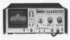
There is a potential personnel and equipment shock hazard in Analyzers with serial numbers 2128A00340 and below. When a new CRT (5083-6176) is installed in these units, approximately 2500 volts is applied via CRT pin 13 (deleted on older CRT's) through the CRT cable assembly and the
